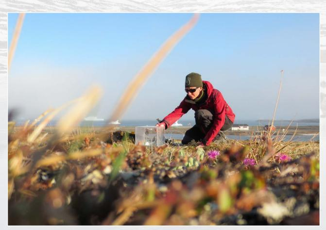
Biogenic volatile organic compounds chamber measurements close to Arctic Station (photo: Frida Lindwall).
