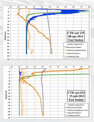
CTD profiles measured at the 'Fast Station'. (A) Spring measurement with algae bloom (i.e., high fluorescence values) and (B) Summer measurement with high surface temperature.
