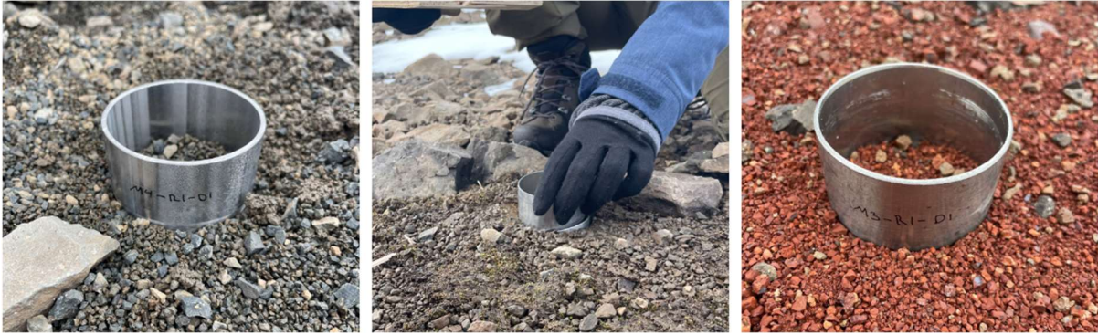
Figure 2 Taking soil samples using steel rings.
